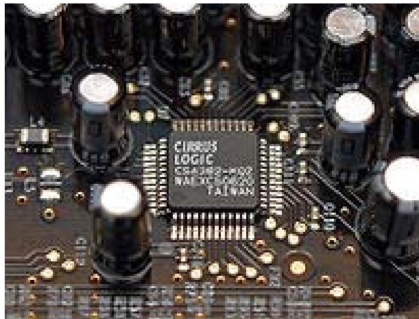
8-channel digital-to-analog converter Cirrus Logic CS4382 placed on Sound Blaster X-Fi Fatal1ty
